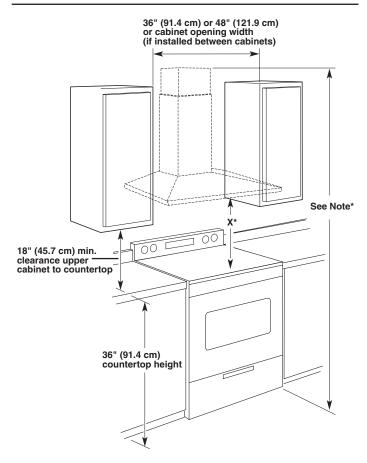
\*NOTE: The range hood chimneys are adjustable and designed to meet varying ceiling or soffit heights depending on the distance "X" between the bottom of the range hood and the cooking surface. For higher ceilings, a 39" (99.1 cm) Chimney Extension Kit Part Number W10197714 (Stainless Steel), is available from your dealer or an authorized parts distributor. The chimney extension replaces the upper chimney shipped with the range hood.
