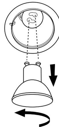
3. Remove the lamp and replace it with a 120-volt, 50-watt maximum halogen lamp with a GU10 base. Turn it clockwise to lock it into place.
