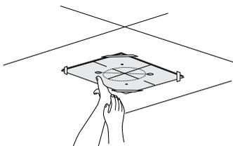
3. Use a pencil to mark the mounting screws, wire access and duct hole locations on the ceiling.
