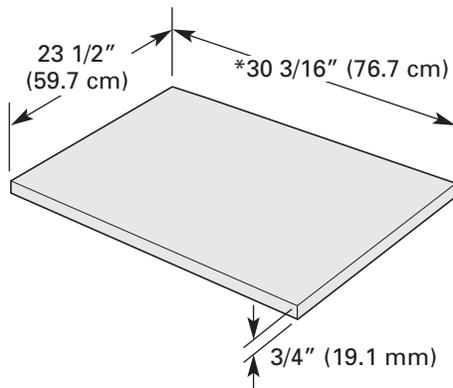
\* This dimension is for 4" (10.2 cm) toe kick. If the installation needs a higher toe kick, adjust the height of the wood panel accordingly. Not recommended for toe kicks greater than 6" (15.2 cm).
