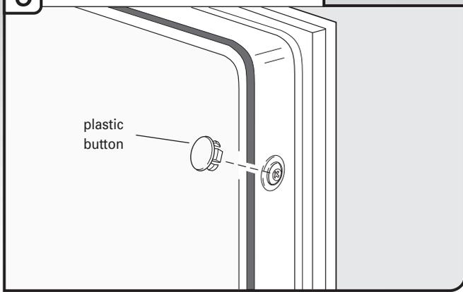
If securing with a side attachment, check that sides of door do not rub against the screw heads. If they do, dishwasher must be re-centered. When dishwasher is properly centered, replace plastic buttons.
