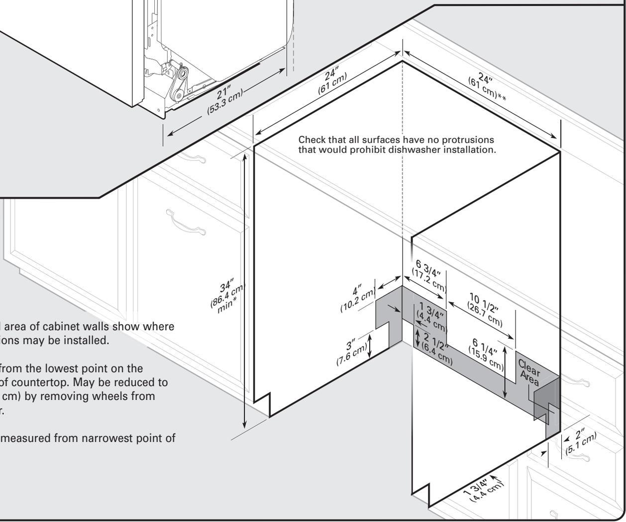
**NOTE:** Shaded area of cabinet walls show where utility connections may be installed.
