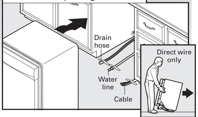
**IMPORTANT:** Double check correct placement of utilities. Grasp the sides of the dishwasher at the edges of the door panel. Tilt dishwasher backwards on wheels and move dishwasher close to cabinet opening.
