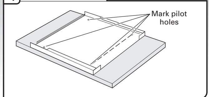
Mark all four hole locations; remove outer panel. Drill 3/32" pilot holes 1/2" (13 mm) deep in customer-supplied custom panel. Place the outer panel on the back of the customer-supplied custom panel; align holes.
