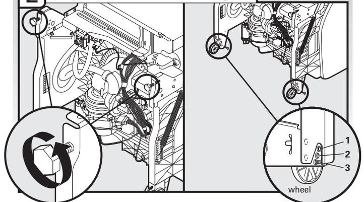
Turn both leveler legs to the same height. Put wheels in the required position determined from "Dishwasher Height Adjustment Chart."
