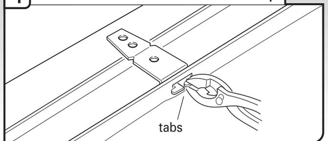
To remove the brackets from the top, flatten tab at back of brackets with pliers, and pull the brackets out of the slots.
