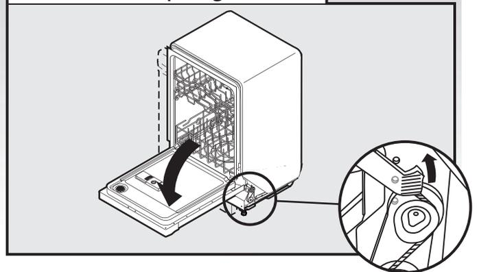
When door is unlatched, and door opens by itself, move the tensioner to a lower numbered hole and replace the screw. Reattach door spring to rear leg.
