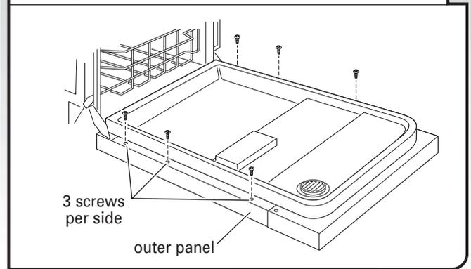
Gently set outer panel aside. Lay the customer-supplied custom panel face down on a covered, non-scratching surface.
