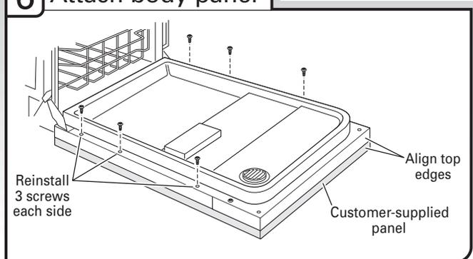
Attach the panel assembly to the door by reinstalling the three screws on each side; do not tighten completely. This reinstallation of the three screws will hold the panel assembly in place on the door frame.
