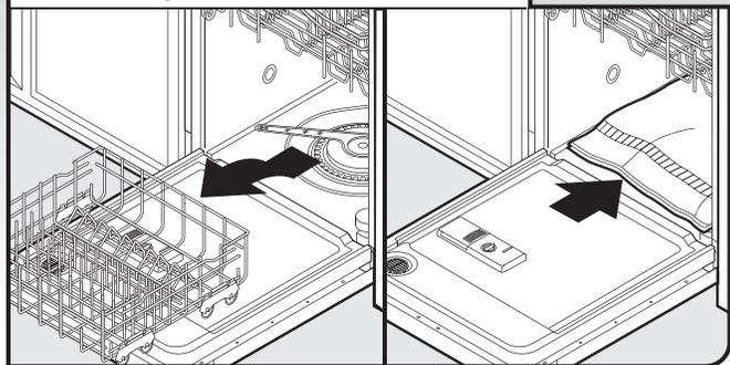
Open dishwasher door, remove lower dish rack, and place towel over pump assembly and lower spray arm of dishwasher. This will prohibit screws from falling into pump area when securing dishwasher to countertop.
