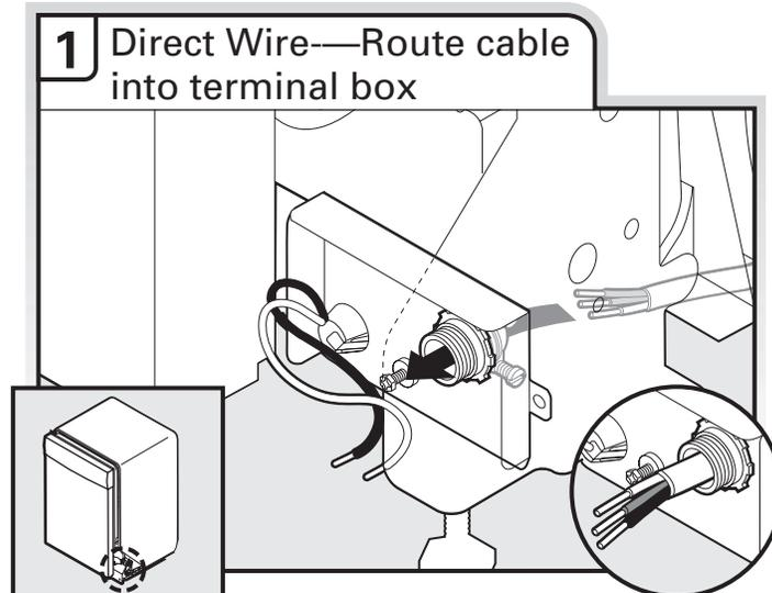
Route cable so that it does not touch dishwasher motor or lower part of dishwasher tub. Pull cable through UL Listed/CSA approved strain relief in terminal box. Strain relief is not supplied with the dishwasher. Owner must purchase a 7/8" screw-in type strain relief.
