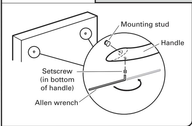
**IMPORTANT:** Do not scratch the front panel during this procedure.
