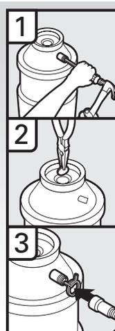
1. Using a hammer and screwdriver, knock plug into disposer.
