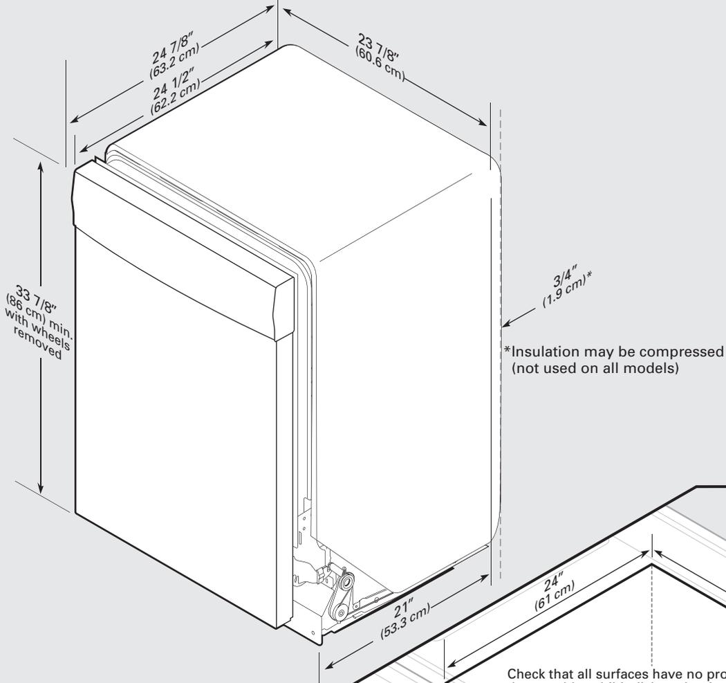
\*Insulation may be compressed (not used on all models)
