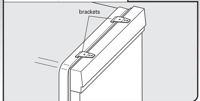
**IMPORTANT:** The dishwasher must be secured to the cabinet. There are two brackets on top of the dishwasher that can be attached to the countertop if it is wood, laminate or other similar surfaces. If your countertop is marble, granite or other hard surface the brackets may be moved to the sides of the dishwasher.
