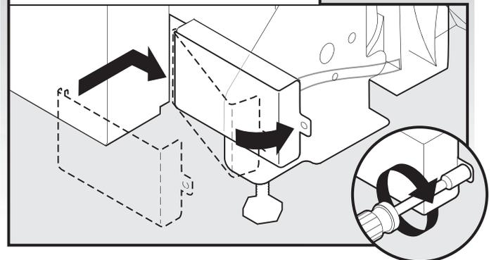
Place wires inside terminal box. Insert tabs on left side of cover. Make sure wires are tucked inside box. Close cover ensuring wires are not pinched. Use 1/4" nut driver and previously removed screw to secure cover.
