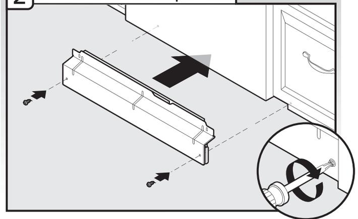
Hold the two panels together and place them against dishwasher leg. Using a Philips or 1/4" screwdriver, reinstall the screws through the holes in the access panel and the slots in the lower panel.
