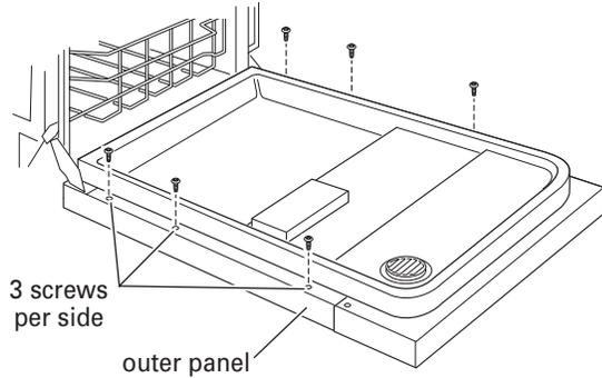
Gently set outer panel aside. Lay the customer-supplied custom panel face down on a non-scratching surface. Position the outer panel on the back of the customer-supplied custom panel as shown; make sure top edge of the outer panel is aligned with the top edge of the customer-supplied custom panel, and both panels are centered side to side.
