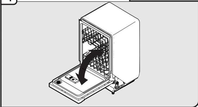
With another person holding the dishwasher to avoid it from tipping, open and close the door a few times. If the door closes or falls open under its own weight, the door tension will need to be adjusted.
