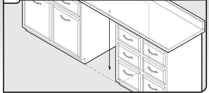
Measure height of cabinet opening from underside of countertop to floor where dishwasher will be installed (you will need to measure the lowest point on the underside of the countertop and the highest point on the floor). Refer to "Dishwasher Height Adjustment Chart" for wheel position and the number of turns needed.
