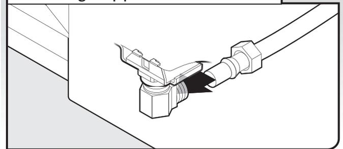
Copper tubing only: Put the tubing into the 90° elbow fitting as far as it will go (the copper tubing bends and kinks easily). Slide the nut and ferrule forward and start the nut onto the elbow threads.
