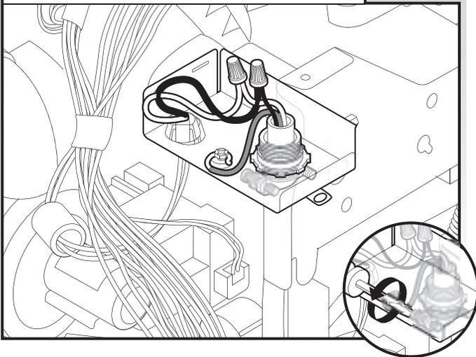
Tighten strain relief screws to secure cord.
