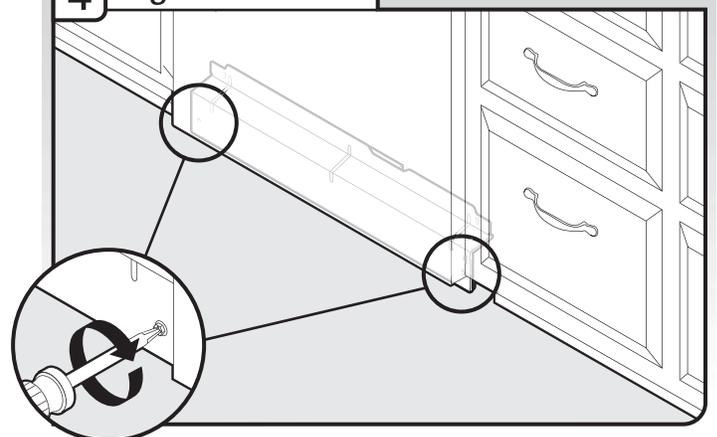
Tighten access panel screws.
