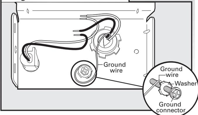
Form bare ground wire into a U-shaped hook. Wrap ground wire hook clockwise around ground connector screw and under the washer. Securely tighten ground connector.
