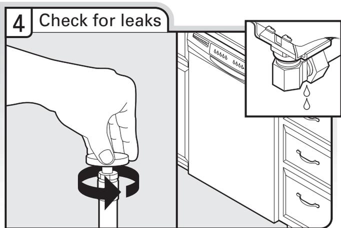
Place paper towel under 90° elbow fitting. Turn on water supply and check for leaks. If leak occurs, repeat previous step.
