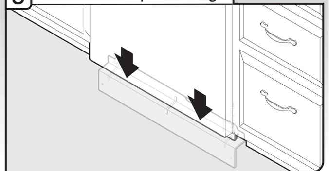
Check that the lower edge of the lower panel contacts the floor. Adjust if necessary.
