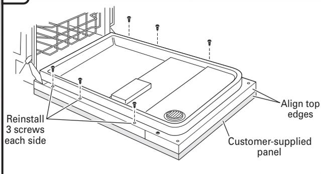
Attach the panel assembly to the door by reinstalling the three screws on each side.
