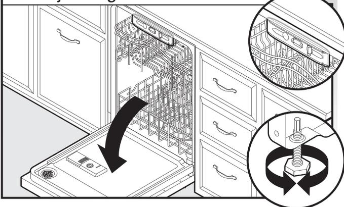
Place level against top front opening of tub. Check that dishwasher is level from side to side. If dishwasher is not level, adjust front legs up or down until dishwasher is level.
