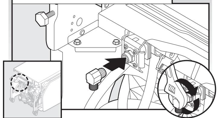
Connect 90° elbow fitting to water inlet valve. Using a wrench, tighten elbow until snug, and be sure that it faces to the rear.
