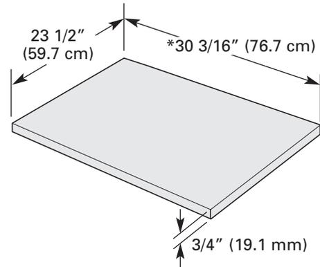
\* This dimension is for 4" (10.2 cm) toe kick. If the installation needs a higher toe kick, adjust the height of the wood panel accordingly. Not recommended for toe kicks greater than 6" (15.2 cm).
