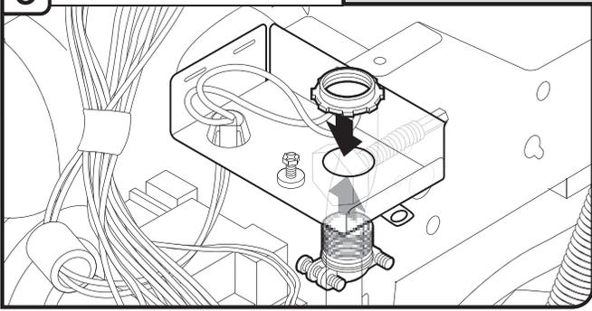
Install a UL listed or CSA approved strain relief. Make sure screwheads are facing to the left when tightening conduit nut. Strain relief is provided with the power supply cord kit.
