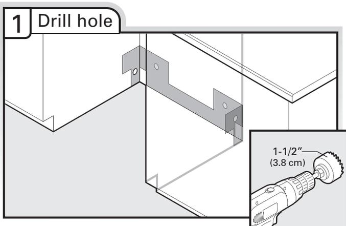
If needed, drill a 1 1/2" (3.8 cm) diameter hole in cabinet wall or side of the opening closest to the sink.
