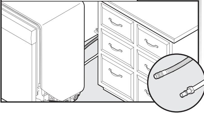
Check that water line is on the left side of opening and drain hose is near the center of the cabinet opening.
