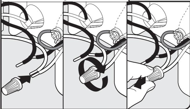
**NOTE:** Twist on UL listed or CSA approved wire connector. Gently tug on wires to be sure both are secured.
