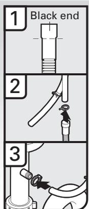
1. Connect black end of drain hose to air gap and cut if needed. (Do not cut ribbed section.)
