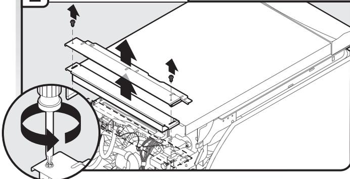
Using a 1/4" hex head socket, nut driver or Phillips screwdriver, remove two screws attaching access panel and lower panel to dishwasher. Do not remove tech sheet from access panel.
