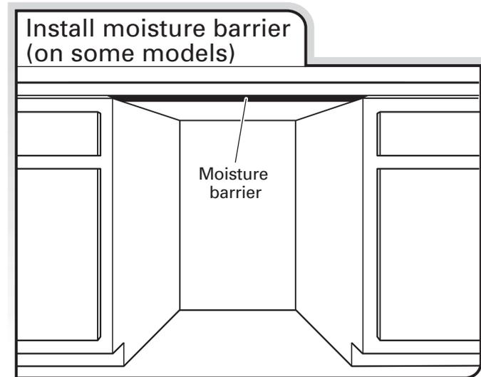
1. Make sure the area under the cabinet is clean and dry for installation of the moisture barrier.
