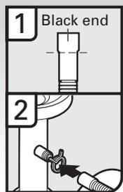
1. Connect black end of of drain hose to waste tee and cut if needed. (Do not cut ribbed section.)
