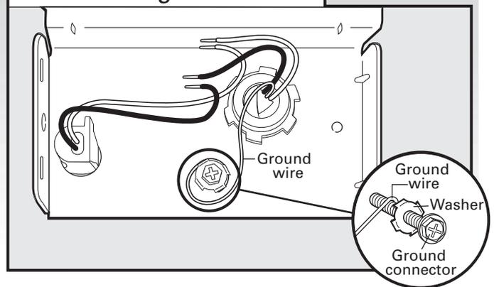
Remove the green grounding screw and place through the ring terminal of the green ground wire. Reattach and tighten the green screw.
