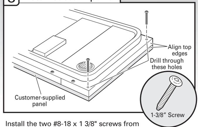
Install the two #8-18 x 1 3/8" screws from the literature package in the top corners of the inner panel. Tighten the six side screws reinstalled in Step 6.
