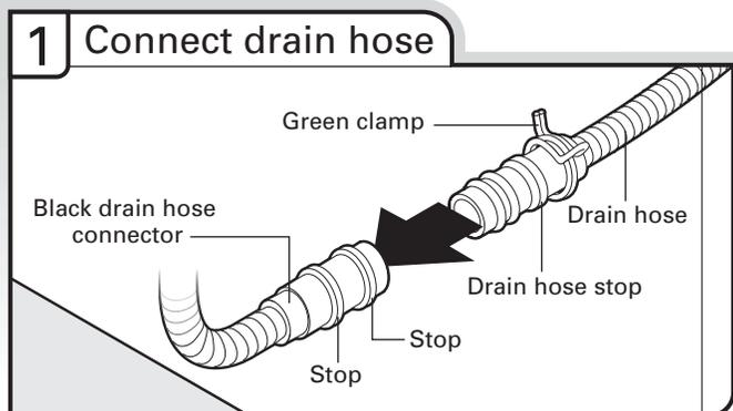
Place towel under drain hose to catch any water in drain hose. Place the small green drain hose clamp onto the small end of the drain hose. Push the new drain hose into the black drain hose connector up to the drain hose stop.
