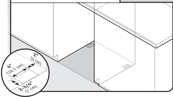
Built-up floors (Kitchen floor height is higher than cabinet opening.) Example: Kitchen floor tile does not extend into cabinet opening. Add shims as needed in the area shown to bring the dishwasher up to 34" (86.4 cm) below the countertop.
