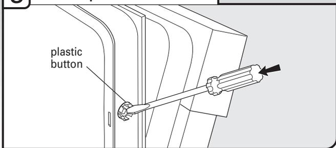
Push the plastic buttons out of the side of the tub.
