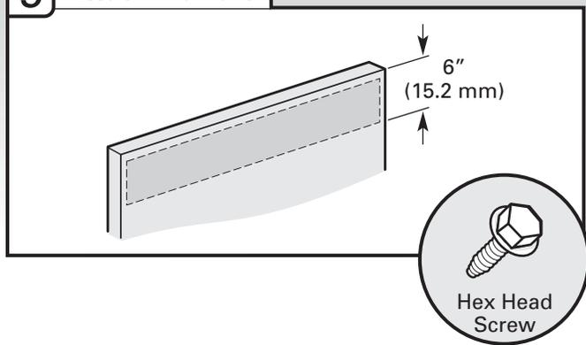
Attach outer panel to back of customer-supplied custom panel with the four #10-16 x 3/8" hex head screws supplied in the literature package. Attach the handle. The handle should be centered on the front of the customer-supplied custom panel in the area shown.
