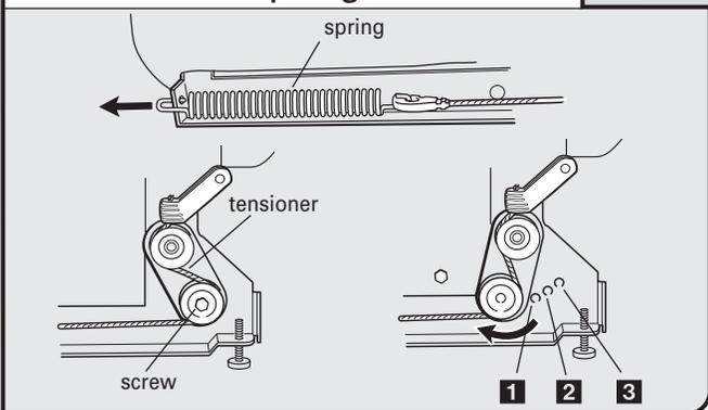
To adjust the door spring tension, unhook the spring from the rear leg of dishwasher. Using a 5/16" nut driver or hex socket, remove the screw from the tensioner.
