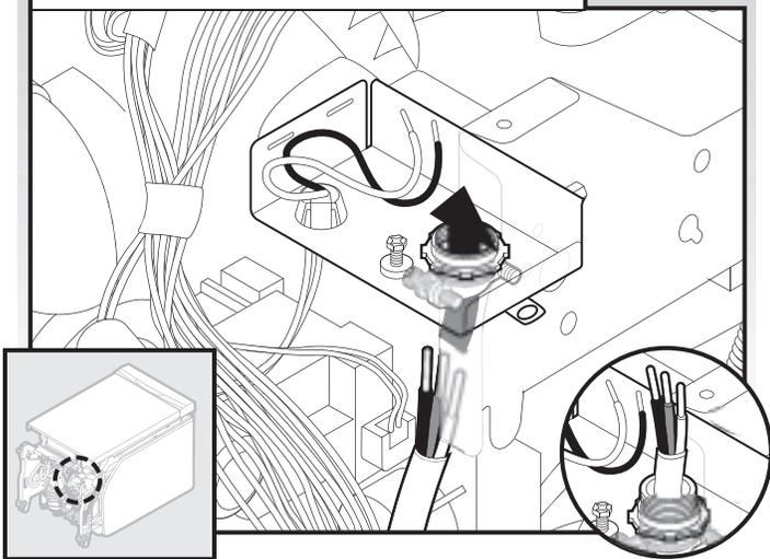
Route cord so that it does not touch dishwasher motor to lower part of dishwasher tub. Pull cord through strain relief in terminal box. Take notice when installing or removing the dishwasher in order to reduce the chance of damaging the power supply cord.
