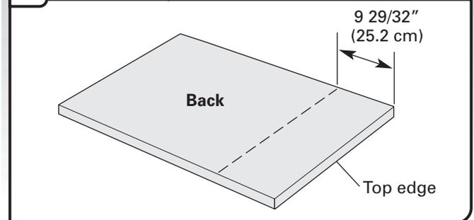
Measure 9 29/32" (25.2 cm) from top edge and mark a line on the back of customer-supplied custom panel. Position the outer panel on the back of the customer-supplied custom panel as shown, so that the top holes in the outer panel are on the line, and both panels are centered side to side.
