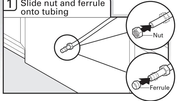
Copper tubing only: Slide nut then ferrule onto copper tubing about 1" (2.5 cm).
