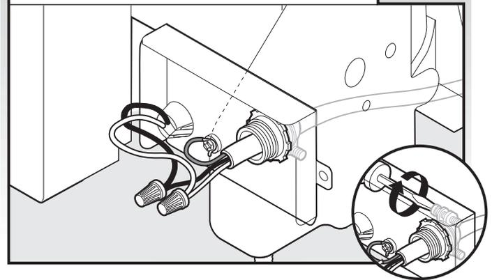
Tighten strain relief screws to secure cable.
