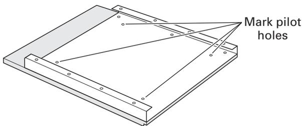
Mark all four hole locations; remove outer panel and drill  $3/32$ " pilot holes  $1/2$ " (13 mm) deep, in customer-supplied custom panel. Place the outer panel on the back of the customer-supplied custom panel and align holes. Attach outer panel to back of customer-supplied custom panel with four #10 x  $1/2$ " wood screws (not supplied). If the customer-supplied custom panel is less than  $3/4$ " (1.9 cm) thick where the screws are attached, shorter screws may be required.
