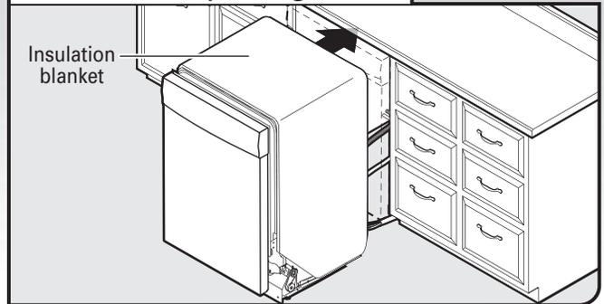
**IMPORTANT:** If wheels were removed, protect the floor when moving the dishwasher. Slowly move dishwasher completely into cabinet opening. Do not kink or pinch water line, drain hose, power supply cord or direct wire between dishwasher and cabinet. Remove cardboard from under dishwasher.
