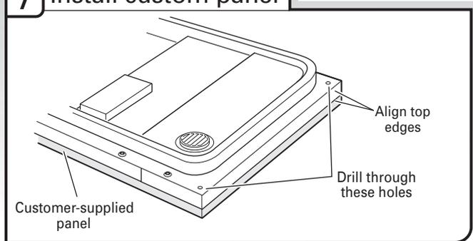
Align the top edge of the customer-supplied custom panel with the top of the console.
