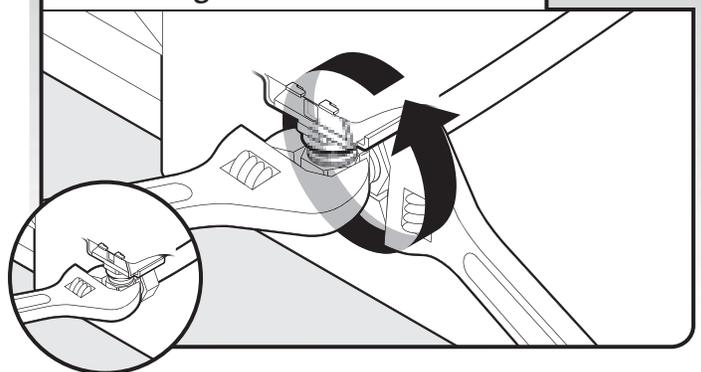
Hold the 90° elbow fitting still with one adjustable wrench and tighten the nut with second adjustable wrench.
