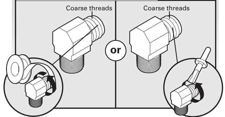
Apply Teflon® tape or pipe joint compound to 90° elbow fitting (not provided). Wrap tape around coarse threads two to four times to prohibit leaks.
