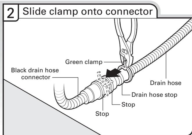
Using pliers, squeeze open the small green drain hose clamp and slide onto connector between stops.
