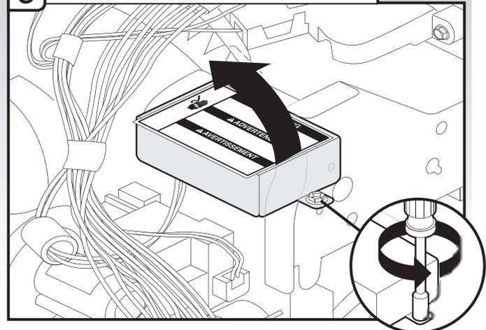
Using a 1/4" hex head socket, nut driver or Phillips screwdriver, remove terminal box cover. Retain for later use.
