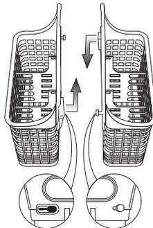
Load the silverware basket while it is in the rack or take the basket out for loading on a counter or table. The silverware basket can be removed for easy unloading.
