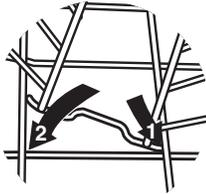
2. Straighten the insert into position along the bottom of the base rack.
