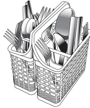
Use the center section with cover down to load silverware in set positions and avoid nesting. Mix items in end sections of the basket with some pointing up and some down to avoid nesting. Spray cannot reach nested items.
