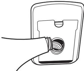
3. Take care not to spill rinse aid into the drawer. Any spills must be wiped up to avoid excess foaming.
