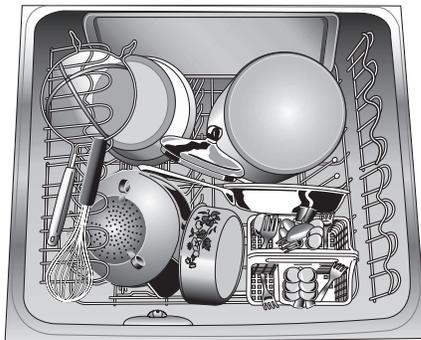
**NOTE:** Do not load items between the rack and the detergent dispenser because they might block the water inlet opening located at the base of the dispenser.
