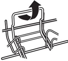
2. Once the handle is lifted up, tilt the insert to the left or right to release the insert legs on the other end from their position under the base rack wire.
