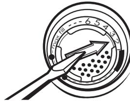
**NOTE:** For most water conditions, the factory setting of 2 will give good results. If you have hard water or notice rings or spots, try a higher setting. Turn the arrow adjuster inside the dispenser by either using your fingers or inserting a flat-blade screwdriver into the center of the arrow and turning.
