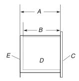
A. 23 <sup>1</sup>⁄<sub>4</sub>" (59.1 cm) min. cutout depth B. 23" (58.4 cm) recessed oven depth C. Oven front D. Recessed oven
