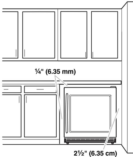
To ensure proper ventilation for your beverage center, allow for a 1/4" (6.35 mm) space on each side and at the top. When installing your beverage center next to a fixed wall, leave 2 1/2" (6.35 cm) minimum clearance on each side to allow for the door to swing open.
