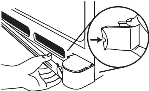
4. Using a screwdriver or  $\frac{3}{8}$ " hex driver, turn the roller adjustment screw(s) on each side to raise or lower that side of the refrigerator.
