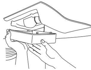
3. Replace burned-out bulb(s) with appliance light bulb(s) no greater than 40 watts.
