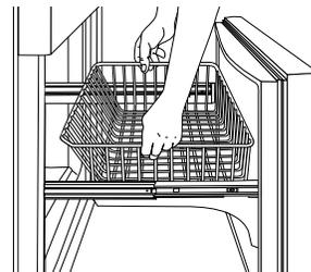
5. Remove the basket cradles from the drawer rails. Push the snap attachments inward away from the drawer rails to unlatch the basket cradles. Lift the basket cradles off the drawer rails.
