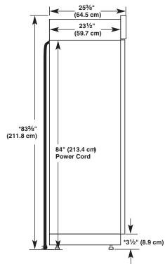
\*When leveling legs are fully extended to 11/4" (3.2 cm) below rollers, add 11/4" (2.9 cm) to the height dimensions.
