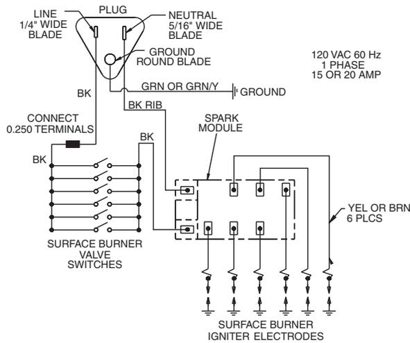
SWITCHES ON SURFACE BURNER VALVES:
