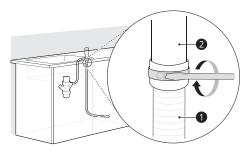
3 If it is not connected, attach the rubber hose connector to the disposal or waste tee with a hose clamp (not provided).
