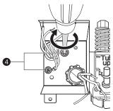
8 Pair the white, black, and green wires to the matching colored wires from the dishwasher. Then twist on the provided wire nuts **5** tightly to connect the corresponding wires.
