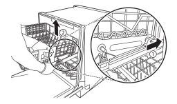
To replace the rack, place the back rack supports behind the rear hooks and pull the rack forward to snap the supports into the hooks. Then align the front rack supports with the front hooks and push the front of the rack down to snap the supports into the front hooks.
