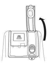
Add a liquid rinse aid to the maximum fill level. Allow the rinse aid to settle in the dispenser while filling, or air bubbles may result in poor drying performance. Avoid overfilling the dispenser.
