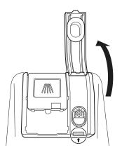
Add a liquid rinse aid to the maximum fill level. Allow the rinse aid to settle in the dispenser while filling, or air bubbles may result in poor drying performance. Avoid overfilling the dispenser.
