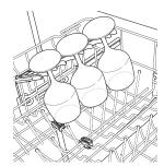
The cup racks can be folded up out of the way for tall glasses.
