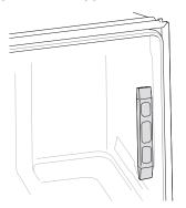
Make sure that the gap between the tub walls and the door liner is the same on either side.
