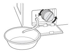
**5** Clean the pump filter and opening.
