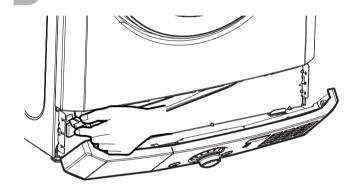
Assemble the control panel by sliding down the panel to the left until it is perfectly fit. (Details on how to connect the control panel is illustrated on next page)
