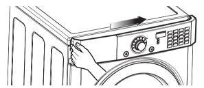
Push the housing hook and disassemble the panel.
