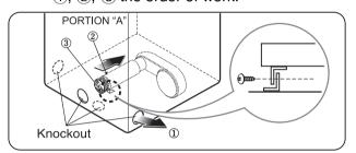
**2-2.** Reconnect the duct to the blower housing and attach the duct to the base.(Duct is a SVC part)
