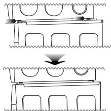
Insert the front stacking kit. Push the front stacking kit back to the stoppers of side
