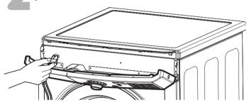
Disassemble the deco by lifting it up slightly.
