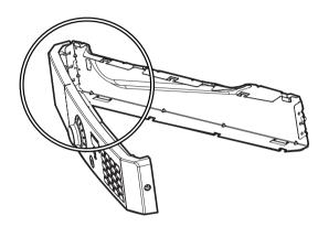
Insert the three of hooks into the holes in the frame and push it inward.
