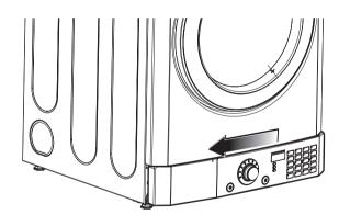
Assemble the lower cover to the upper side of the machine.
