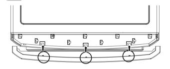
Insert the four of hooks into the holes in the frame and push it inward.
