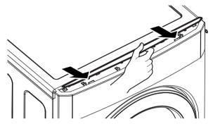
Assemble the upper deco by sliding it down to the left.
