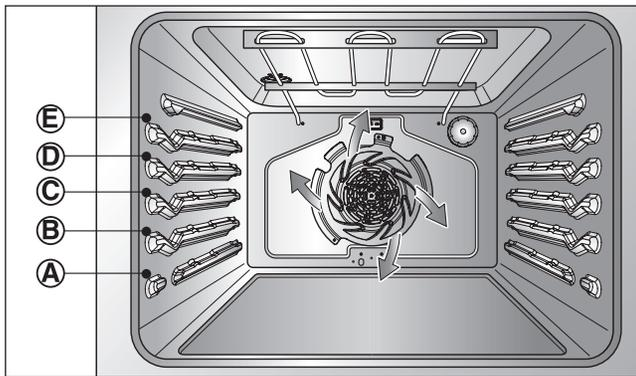
The **CONV. BAKE** pad controls the Convection Bake feature. Use the Convection Bake feature when cooking speed is desired. The oven can be programmed for Convection Bake at any temperature between 300°F (150°C) to 550°F (285°C).
