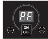
If a flashing time is in the display, you have experienced a power failure. Reset the clock. Touch the **CLOCK** pad once to reset. Enter the correct time of day by touching the appropriate number pads. Touch the **START** pad.
