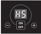
The display will Flash HS(Hot Surface). When the surface is too hot to touch because of the heating element. It will remain on after the element is turned off and the surface has cooled to approximately 150 deg F.
