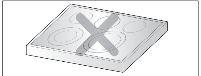
During a self clean cycle in either the upper or lower oven the cooktop elements can not be used. If running a self clean in one of the ovens the other oven can not be used. Self clean can only be run in one oven at a time.
