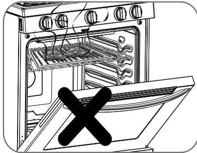
**NOTE:** If the oven door remains open for more than 15 seconds during broil the burner will shut off. The broil burner will automatically come back on once the door is closed.
