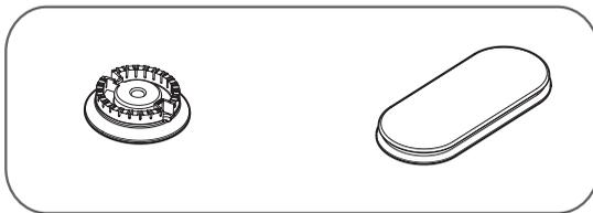
The burner heads and the oval burner head/cap assembly are removable. Simply lift them off the range for cleaning. For even and unhampered flame, the slits in the burner heads must be kept clean at all times. Clogged or dirty burner ports or electrodes will not allow the burner to operate properly. Any spill on or around an electrode must be carefully cleaned. Take care to not hit an electrode with anything hard or it could be damaged.
