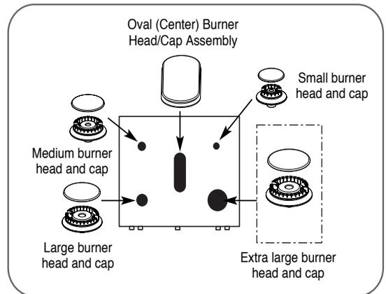
Make sure the hole in the burner head is positioned over the electrode.
