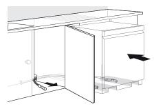
**5** Remove the tape from the water supply line and the electrical cable.
