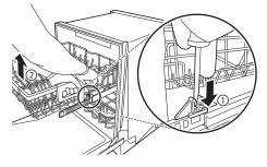
**3** To remove the back rack supports from the rails, hold a side rail with one hand, lift the front of the rack, and firmly push the rack back to snap the support out of the hooks in the rear. Repeat on the opposite side.
