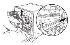
4 To replace the rack, place the back rack supports behind the rear hooks and pull the rack forward to snap the supports into the hooks. Then align the front rack supports with the front hooks and push the front of the rack down to snap the supports into the front hooks.
