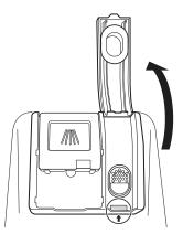
**2** Add a liquid rinse aid to the maximum fill level. Allow the rinse aid to settle in the dispenser while filling, or air bubbles may result in poor drying performance. Avoid overfilling the dispenser.
