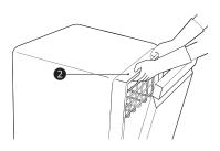
Align the dishwasher with the opening. Make sure the water supply line and electrical cable are in the correct positions to slide into their channels properly.
