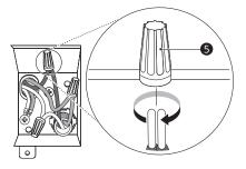
**9** Wrap electrical tape **6** around each connection.
