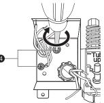
8 Pair the white, black, and green wires to the matching colored wires from the dishwasher. Then twist on the provided wire nuts **9** tightly to connect the corresponding wires.
