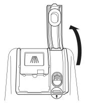
**2** Add a liquid rinse aid to the maximum fill level. Allow the rinse aid to settle in the dispenser while filling, or air bubbles may result in poor drying performance. Avoid overfilling the dispenser.
