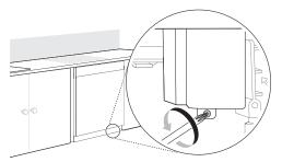
3 Use a Phillips screwdriver to remove 2 screws ●.
