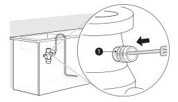
**2** Remove the knockout plug **1** from the disposal.
