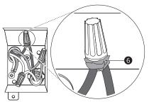
**10** Fold the connected wires back into the junction box and screw on the junction box cover.
