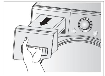
2. Using the handle on the front of the drawer, pull out the reservoir.
