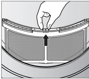
3. Open the filter and use your fingers to roll the lint off the screen surfaces. If the lint is difficult to remove or the filter material is showing signs of clogging, follow the cleaning instructions below.
