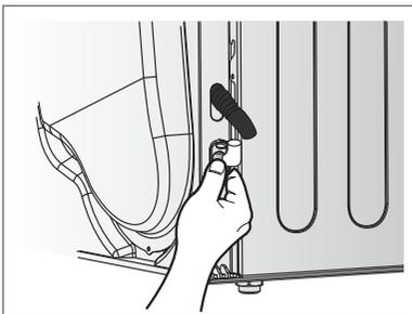
3. Connect the external drain hose included with the dryer. Route this hose to a permanent drain and secure the hose so it can not come loose.
