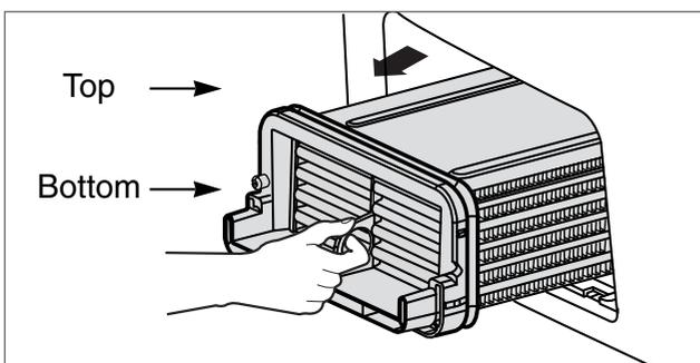
4. Thoroughly clean the condenser by running tap water through it from both the ends and the sides.
