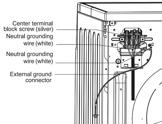
1. Connect neutral wire (white) of power cord to center terminal block screw.
