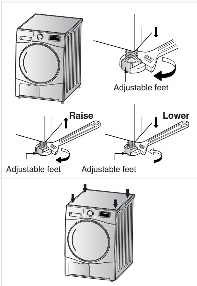
2. If the dryer is not properly level, adjust the front leveling legs up and down as necessary.
