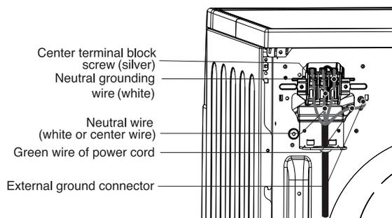
1. Connect neutral wire (white) of power cord to center terminal block screw.
