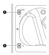
2 While supporting the door, remove the 2 screws 2 on the door hinge, two from each hinge. Set the door aside face down on a protected surface to prevent damage to the door or the work surface.
