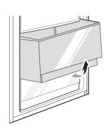
Press on the hook inside the top compartment, and then take out the air filter.
