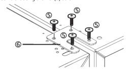
**6.** Remove the No. (5) screw from the bottom of the front of the product. Align the No. (2) bracket frame with the hole in the product and reassemble it using the No. (5) screw.
