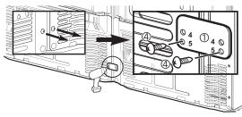
**5.** Align the No. (6) bracket frame with the hole in the top of the product and assemble it using the No. (5) screw.
