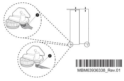
**4.** Remove the No. (4) screw from the radiation grill in the back of the product. Align the No. (1) bracket frame in the hole in the product and reassemble it using the No. (4) screw.
