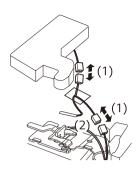
3 Rotate the hinge lever counterclockwise. Lift the top hinge free of the hinge lever latch.
