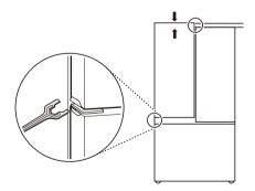
The right refrigerator door does not have an adjustable nut.
