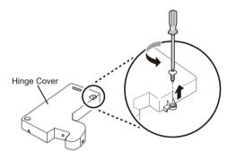
**2** Disconnect all the wire harnesses (1). Unscrew the ground wire (2).
