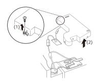
2 Disconnect all the wire harnesses (1). Unscrew the ground wire (2).
