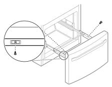
4 Insert the drawer into the frame, and push the drawer back until it clicks into place.
