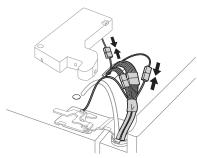
Push the water supply tube into the hole on the top case and pull it through the backplate.
