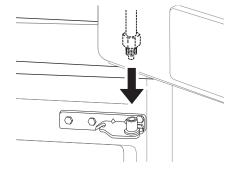
Fit the hinge **1** over the hinge lever latch **2** and slot it into place. Rotate the lever 3 counterclockwise to secure the hinge.
