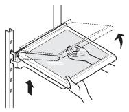
To assemble, tilt the front of the shelf up and guide the shelf hooks into the slots at a desired height.
