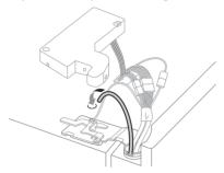
Hold the water supply connection and gently push in the collet 4 to connect the water supply line as shown. Insert the tube at least 5/8 inch (15 mm) into the connector. Insert the clip on the joint to fasten the tube in place.
