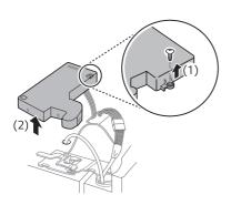
3 Remove the cover and pull out the tube (1). Disconnect all wire harnesses (2). Unscrew the ground wire (3).
