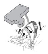
**4** Rotate the hinge lever counterclockwise (1). Lift the top hinge (2) free of the hinge lever latch.
