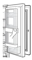
To remove the case, lift up and pull out.
