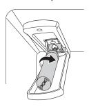
Close the water filter cover. The cover will click when closed correctly.
