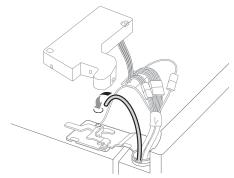
**5** Hold the water supply connection and gently push in the collet 4 to connect the water supply line as shown. Insert the tube at least 5/8 inch (15 mm) into the connector. Insert the clip on the joint to fasten the tube in place.
