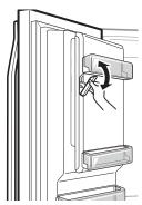
To remove the in-door ice bin, grip the front handle, slightly lift the lower part, and slowly pull out the bin as shown.
