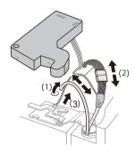
Rotate the hinge lever counterclockwise (1). Lift the top hinge (2) free of the hinge lever latch.
