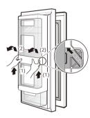
2 To replace the Door-in-Door case, line up the tabs on the Door-In-Door case with the slots on the door and push down until it snaps into place.
