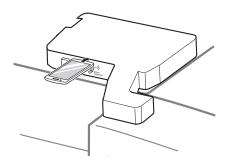
Press and hold the Freezer button for three seconds while continuing to hold your phone to the speaker.
