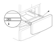
4 Insert the basket into the frame, and push the drawer back until it clicks into place.
