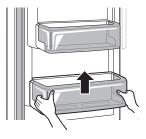
To assemble the bin, slide it in above the desired support and push down until it snaps into place.
