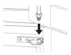
Fit the hinge **1** over the hinge lever latch **2** and slot it into place. Rotate the lever 3 counterclockwise to secure the hinge.
