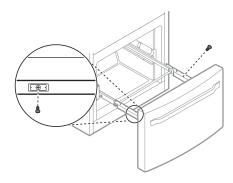
Insert the drawer into the frame, and push the drawer back until it clicks into place.
