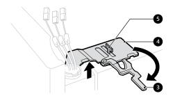
Lift the door from the middle hinge pin and remove the door.
