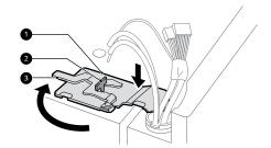
Connect all the wire harnesses and the ground wire.
