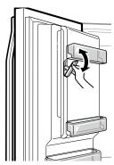
2 To remove the in-door ice bin, grip the front handle, slightly lift the bottom, and slowly pull out the bin as shown.
