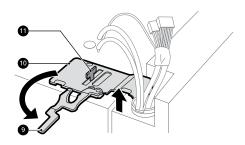
Lift the door from the middle hinge pin and remove the door.
