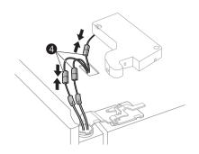
4 Place the cover **(**) in its place. Insert and tighten the cover screw **(**).
