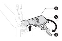
4 Lift the door from the middle hinge pin and remove the door.
