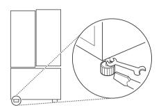
2 Open both doors and check to make sure that they close easily. If the doors do not close easily, tilt the refrigerator slightly more to the rear by turning both leveling legs to the left. It may take several more turns, and be sure to turn both leveling legs the same amount.
