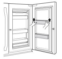
**2** To replace the door bins, slide the door bin in above the desired support and push down until it snaps into place.
