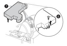
3 Remove the cover and pull out the tube <sup>(3)</sup>. Disconnect all wire harnesses <sup>(9)</sup>. Unscrew the ground wire <sup>(10)</sup>.
