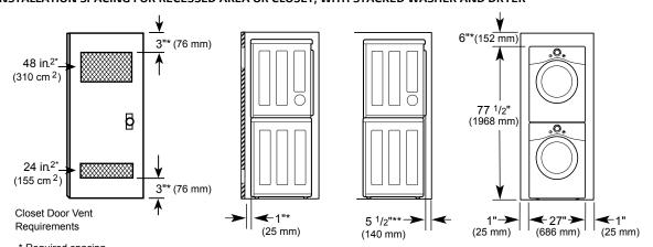
INSTALLATION SPACING FOR RECESSED AREA OR CLOSET, WITH STACKED WASHER AND DRYER
