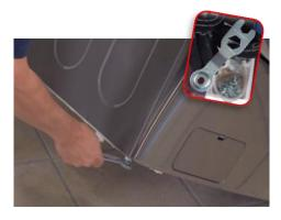
→ Using the wrench provided make sure the legs of the FLW are fully retracted and level prior to mounting
