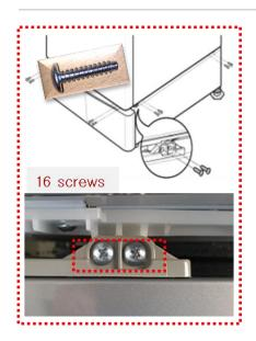
→ Secure FLW to Sidekick with 16 screws provided. Not using all screws can cause noise and vibration issues.
