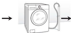
Connecting the drain line
