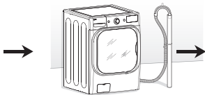
Connecting the drain line
