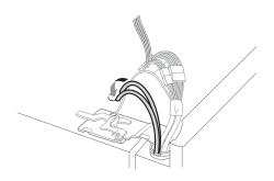
Hold the water supply connection and gently push in the collet **4** to connect the water supply lines as shown. Insert the tube at least 5/8 inch (15 mm) into the connector. Insert the clip on the joint to fasten the tubes in place.
