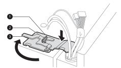
Connect all the wire harnesses and the ground wire.
