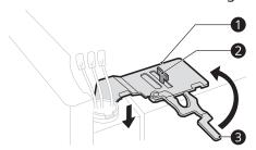
3 Connect all the wire harnesses 4. Screw in the ground wire 5.
