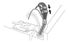
Push the water supply lines into the hole on the top case and pull them through the backplate.
