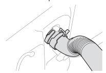
Adjust the band clamp with pliers to keep the hose securely in place and prevent leaking.
