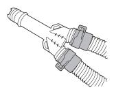
3 Insert the end of the drain hose connector into the laundry tub or standpipe. Use the band clamps to keep it in place, if needed.
