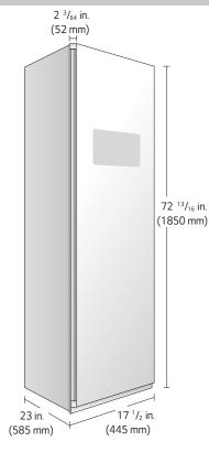
The following clearances are recommended for the Styler. The Styler has been tested for clearances of 13/16 inch (3 cm) on the sides and rear.
