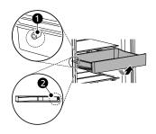
**2** Tilt the drawer slightly and support it with one hand while pulling it out.
