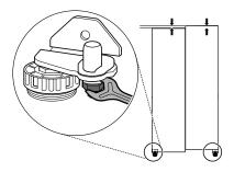
1 Open the door and use the wrench ● to loosen the keeper nut by turning it to the left.
