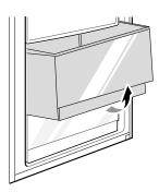
**2** To reassemble, slightly tilt up the front, insert the crisper into the frame and push it back into place.
