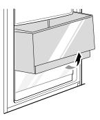
**2** Press on the hook inside the top compartment, and then take out the air filter.
