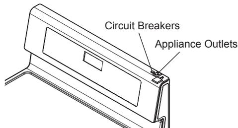
The 120V appliance outlets located on the control console may be used to run portable appliances placed on countertops beside the range. The outlets operate independently and are not affected by range control settings.
