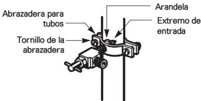
6 ENCAMINE LA TUBERÍA.
