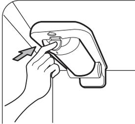
**NOTE:** Replacing the water filter causes a small amount of water (around 1 oz. or 25 cc) to drain. Place a cup under the front end of the water filter cover to collect any leaking water. Hold the water filter upright, once it is removed, to prevent any remaining water from spilling out of the water filter.
