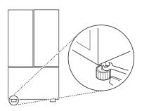
Open both doors and check to make sure that they close easily. If the doors do not close easily, tilt the refrigerator slightly more to the rear by turning both leveling legs to the left. It may take several more turns, and be sure to turn both leveling legs the same amount.
