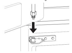
Fit the hinge **1** over the hinge lever latch **2** and slot it into place. Rotate the lever 3 clockwise and fasten the hinge.
