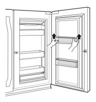
To replace the door bins, slide the door bin in above the desired support and push down until it snaps into place.
