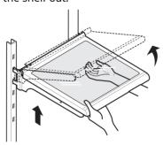
To assemble, tilt the front of the shelf up and guide the shelf hooks into the slots at a desired height.
