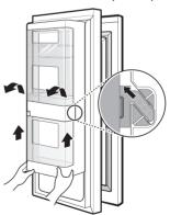
To replace the case, line up the tabs on the case with the slots on the door and push down until it snaps into place.
