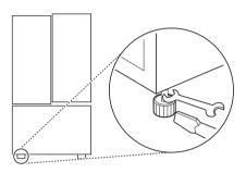
2 Open both doors and check to make sure that they close easily. If the doors do not close easily, tilt the refrigerator slightly more to the rear by turning both leveling legs to the left. It may take several more turns, and be sure to turn both leveling legs the same amount.
