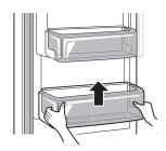
To assemble the bin, slide it in above the desired support and push down until it snaps into place.
